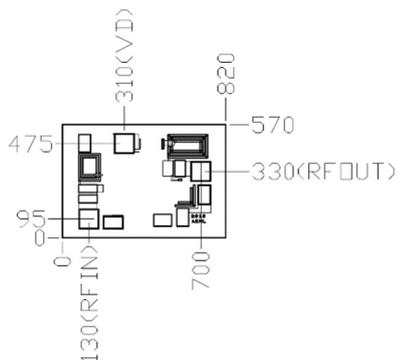
t=100 μm, Pads size 90x90 μm<sup>2</sup>
